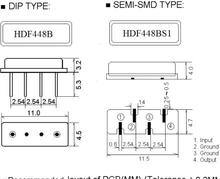
Recommended layout of PCB(MM) (Tolerance ± 0.2MM) for Semi-SMD TYPE |1.1|
