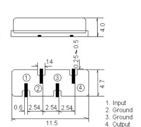
■Recommended layout of PCB(MM) (Tolerance ± 0.2MM)
