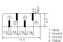
■Recommended layout of PCB(MM) (Tolerance ± 0.2MM)
