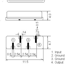
■Recommended layout of PCB(MM) (Tolerance ± 0.2MM)
