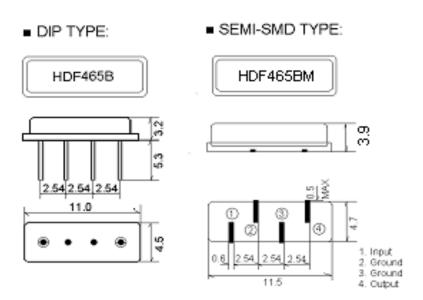
■Recommended layout of PCB(MM) (Tolerance ± 0.2MM)
