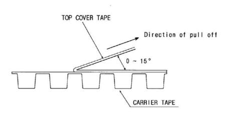
[Figure 1] Carrier Tape Dimensions
