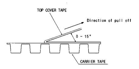
[Figure 1] Carrier Tape Dimensions
