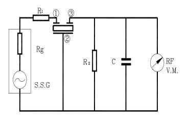
$Rg+R1=R2=1000 \Omega$  (Input/Output Impedance) C=10 pF (Including stray capacitance and input capacitance of RF voltmeter)
