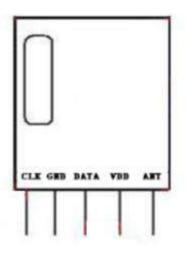
Figure1 TX3-V2.0 Shape & Pins
