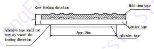
Connect the back face of tapes together with a adhesive tape. Total thickness of tape 1.05mm max.
