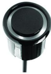
An assembled ultrasonic sensor is a specially assembled unit for parking assistant system consists of pure sensor, rubber ring, plastic shell and cable. It is a key component of reversing radar and can be connected with the signal processing module directly.
