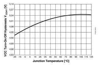
Figure 28 VCC Turn-On/Off Hysteresis  $V_{VCCHY}$  vs.  $T_j$
