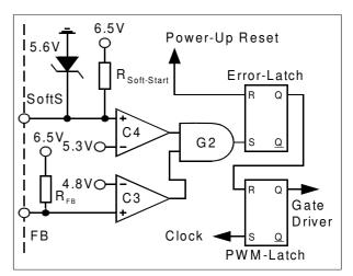
Figure 10 Activation of Protection Unit
