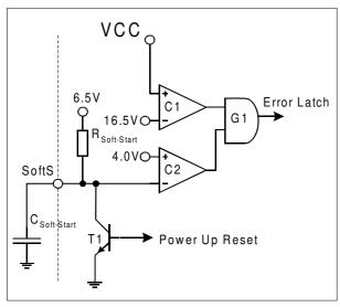
Figure 22 Overvoltage Detection
