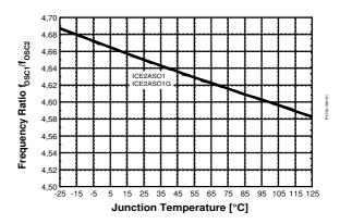
Figure 34 Frequency Ratio  $f_{OSC1}/f_{OSC2}$  vs.  $T_i$
