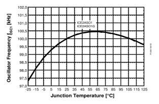
Figure 30 Oscillator Frequency  $f_{OSC1}$  vs.  $T_j$
