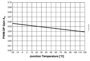
Figure 37 PWM-OP Gain  $A_V$  vs.  $T_i$
