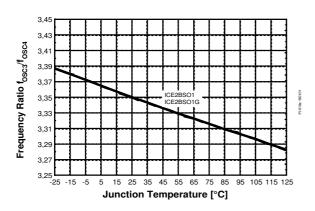
Figure 35 Frequency Ratio  $f_{OSC3}/f_{OSC4}$  vs.  $T_i$
