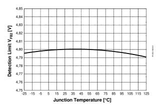
Figure 40 Detection Limit  $V_{FB2}$  vs.  $T_i$
