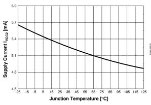
Figure 24 Supply Current  $I_{VCC2}$  vs.  $T_i$
