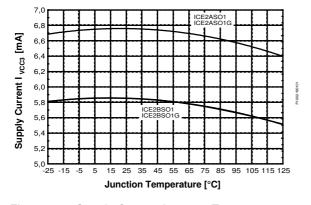
Figure 25 Supply Current  $I_{VCC3}$  vs.  $T_j$
