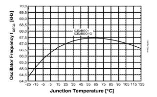
Figure 31 Oscillator Frequency  $f_{OSC3}$  vs.  $T_i$
