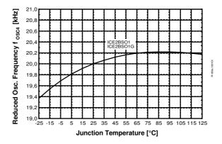
Figure 33 Reduced Osc. Frequency f<sub>OSC4</sub> vs. T<sub>i</sub>
