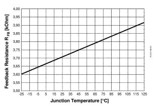
Figure 38 Feedback Resistance  $R_{FB}$  vs.  $T_i$
