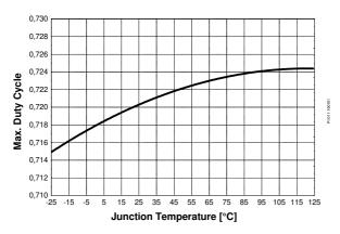
Figure 36 Max. Duty Cycle vs. T<sub>i</sub>
