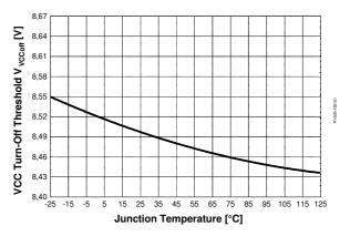
Figure 27 VCC Turn-Off Threshold V<sub>VCCoff</sub> vs. T<sub>i</sub>
