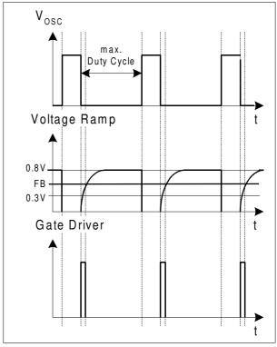
Figure 7 Light Load Conditions
