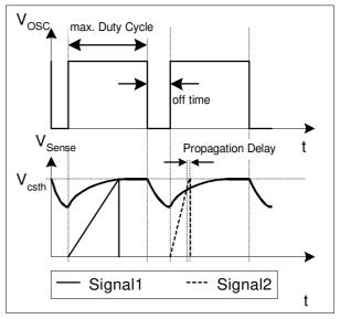
Figure 15 Dynamic Voltage Threshold V<sub>csth</sub>
