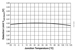
Figure 42 Detection Limit V<sub>Soft-Start2</sub> vs. T<sub>i</sub>
