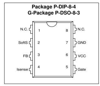
**Figure 1** Pin Configuration (top view)
