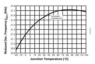
Figure 32 Reduced Osc. Frequency  $f_{OSC2}$  vs.  $T_j$
