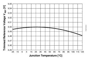
Figure 29 Trimmed Reference  $V_{REF}$  vs.  $T_i$
