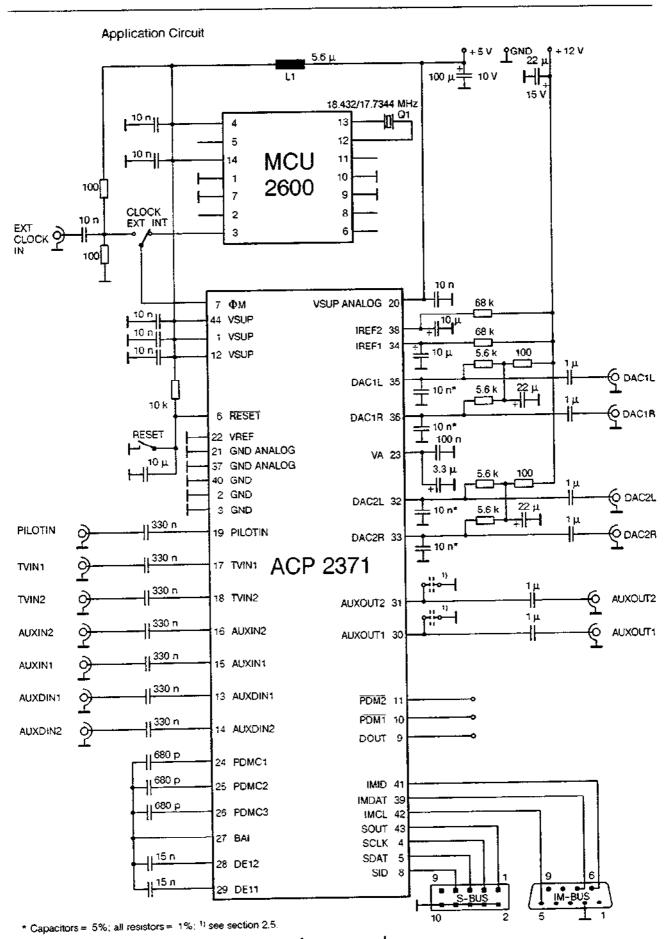
Fig. 6: Digital Audio Appl. circuit
