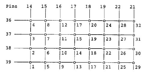
Fig. 1: Diagram of the keyboard for direct input
