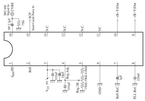
Note) The following signal is inputted to Pin1 from the AN5192/95.
