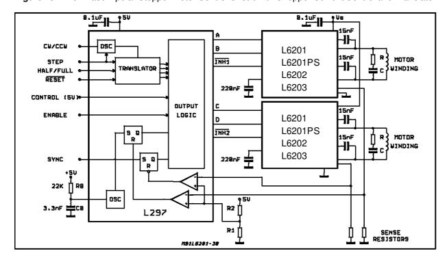
It could be requested to drive a motor at  $V_{\rm S}$  lower than the minimum recommended one of 12V (See Electrical Characteristics); in this case, by accepting a possible small increas in the RDS (ON) resistance of the power output transistors at the lowest Supply Voltage value, may be a good solution the one shown in Fig. 20.
