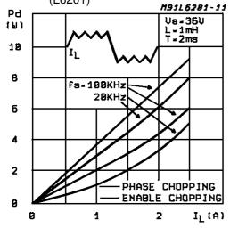
**Figure 6b:** Typical Diode Behaviour in Synchronous Rectification (L6201PS/02/03)
