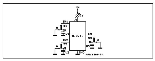
Figure 11: Leakage Current
