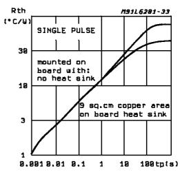
Figurre 23: Typical R<sub>Th J-amb</sub> vs. Two "On Board" Square Heatsink (L6202)
