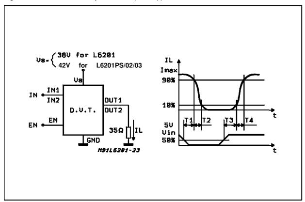
Figure 13: Sink Current Delay Times vs. Input Chopper
