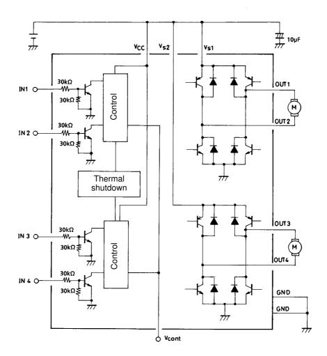
Note: As long as the voltages applied to  $V_{CC}$ ,  $V_S1$ ,  $V_S2$ , and IN1 through IN4 are within the limits set by the absolute maximum ratings, there are no restrictions on the relationship of each voltage level in comparison with the others (regarding which is higher or lower). (ex.  $V_{CC}=3$  V,  $V_S1$ , Z=2 V, IN1 to IN4 = 5 V)
