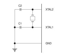
Note: C1, C2 = 30 pF  $\pm$  10 pF for Crystals = 40 pF  $\pm$  10 pF for Ceramic Resonators
