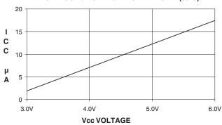
Power-Down Mode Notes: 1. XTAL1 tied to GND for  $I_{CC}$  (power-down) 2. P.1.0 and P1.1 =  $V_{CC}$  or GND 3. Lock bits programmed
