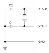
Note: C1, C2= 30 pF  $\pm$  10 pF for Crystals = 40 pF  $\pm$  10 pF for Ceramic Resonators
