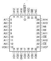
VSOP Top View (8 x 14 mm) or TSOP Top View (8 x 20 mm) **Type 1**
