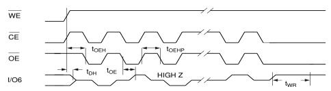
Notes: 1. Toggling either  $\overline{OE}$  or  $\overline{CE}$  or both  $\overline{OE}$  and  $\overline{CE}$  will operate toggle bit. The  $t_{OEHP}$  specification must be met by the toggling input(s).
