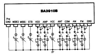
Figure 3 Ripple rejection rate test circuit
