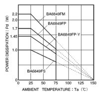
Fig.14 Package derating characteristics
