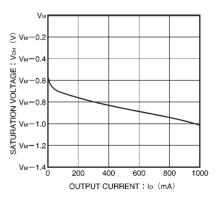
Fig.16 Upper-side output saturation voltage vs. output current
