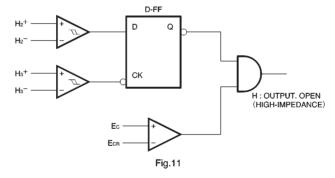
The reverse detection circuit construction is shown in Fig.11.
