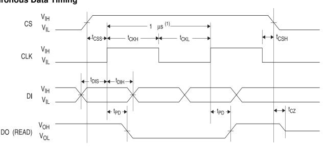
Timing Diagrams Synchronous Data Timing
