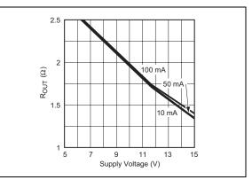
FIGURE 2-12: Low-State Output Resistance vs. Supply Voltage.
