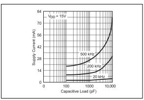
FIGURE 2-6: Capacitive Load.
