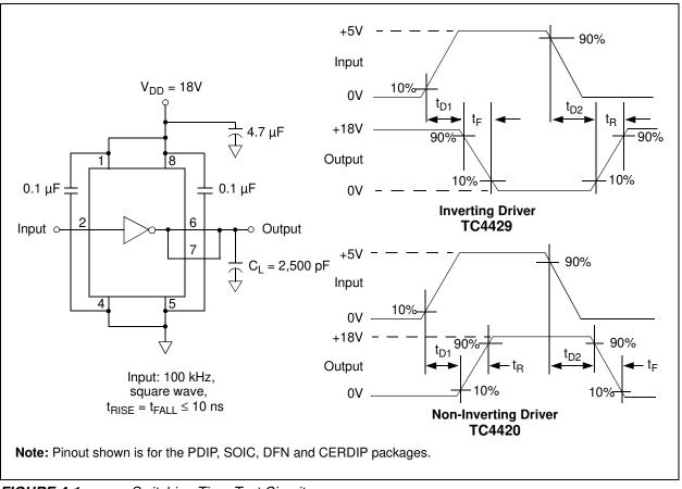
FIGURE 4-1: Switching Time Test Circuits.
