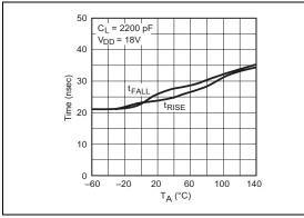
FIGURE 2-7: Rise and Fall Times vs. Temperature.
