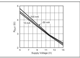
FIGURE 2-10: High-State Output Resistance vs Supply Voltage.
