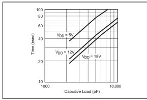
FIGURE 2-2: Rise Time vs. Capacitive Load.
