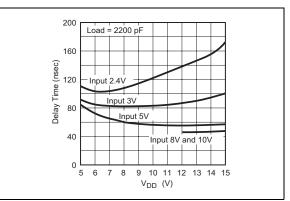
**FIGURE 2-11:** Effect of Input Amplitude on Propagation Delay.
