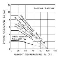
Fig.8 Power dissipation curves (BA6238A/BA6239A)
