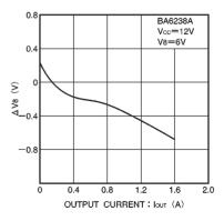
Fig.16 Pin-8 voltage variation vs. output current
