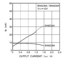
Fig.14 Pin-8 current vs. output current
