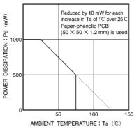
Fig.9 Power dissipation curve (BA6238AN/BA6239AN)
