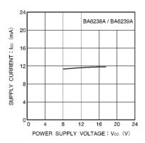
Fig.10 Supply current vs. power supply voltage
