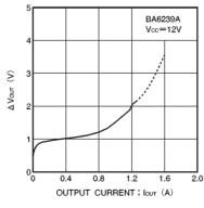
Fig.15 Output voltage variation vs. output current
