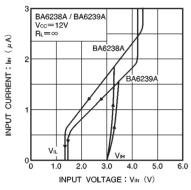
Fig.11 Input current vs. input voltage
