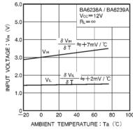
Fig.12 Input voltage vs. ambient temperature
