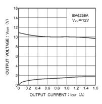
Fig.17 Output voltage vs. output current (BA6238A)
