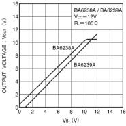
Fig.13 Output voltage vs. pin-8 voltage
