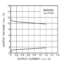
Fig.18 Output voltage vs. output current (BA6239A)
