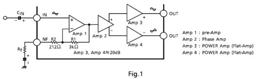
This IC has the amplifier construction as shown in Fig.1. The pre-amp (amp 1) is provided to the primary stage, and the input voltage is amplified by the flat amps, amp 3 and amp 4 of each channel through the phase amp. (Amp 2).
