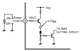
Fig.3 With pin(4) set to high, power is on.
