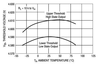
Figure 4. Comparator Threshold Voltage versus Temperature
