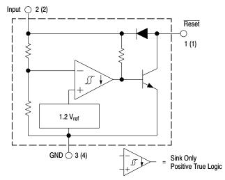
Pin numbers adjacent to terminals are for the 3-pin TO-92 package. Pin numbers in parenthesis are for the 8-lead packages.
