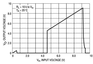
Figure 2. Reset Output Voltage versus Input Voltage
