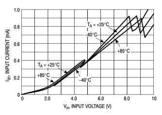
Figure 5. Input Current versus Input Voltage
