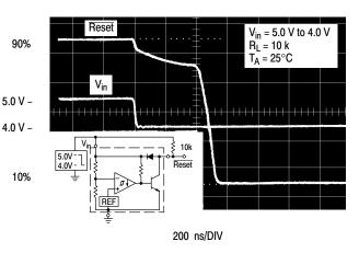
Figure 7. Reset Delay Time
