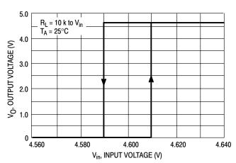
Figure 3. Reset Output Voltage versus Input Voltage
