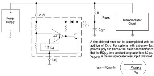
Figure 9. Low Voltage Microprocessor Reset
