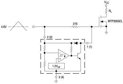
Overheating of the logic level power MOSFET due to insufficient gate voltage can be prevented with the above circuit. When the input signal is below the 4.6 V threshold of the MC34064, its output grounds the gate of the  $\rm L^2$  MOSFET.
