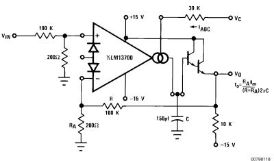
Voltage Controlled Low-Pass Filter
