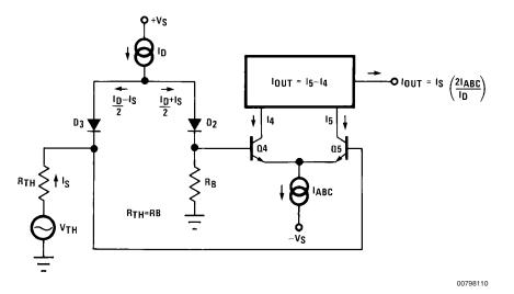
FIGURE 3. Equivalent VCA Input Circuit
