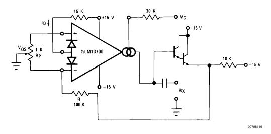
FIGURE 9. Voltage Controlled Resistor with Linearizing Diodes
