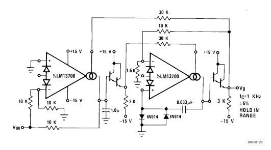
FIGURE 21. Phase Lock Loop
