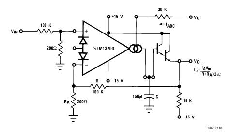
FIGURE 11. Voltage Controlled Low-Pass Filter
