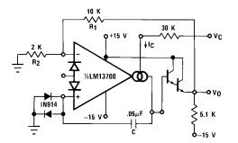
Figure 18 shows how to build a VCO using one amplifier when the other amplifier is needed for another function.
