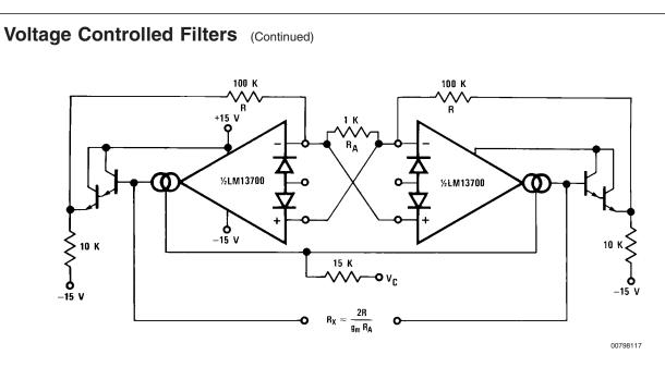
FIGURE 10. Floating Voltage Controlled Resistor
