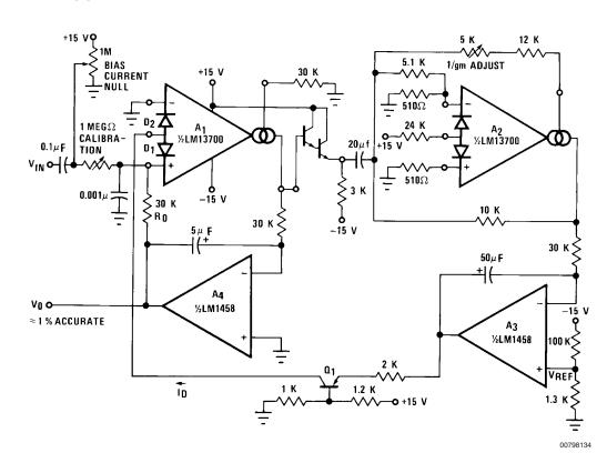
FIGURE 27. True RMS Converter
