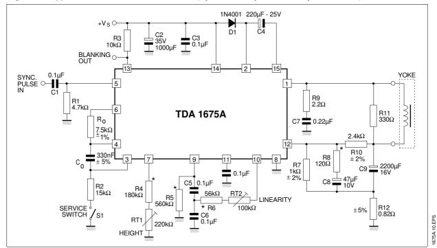
Figure 5 : Application Circuit for  $110^{\circ}$  CTV Set (R<sub>y</sub> =  $5.9\Omega$  ; L<sub>y</sub> = 10 mH ; I<sub>y</sub> = 1.95 A<sub>PP</sub>)
