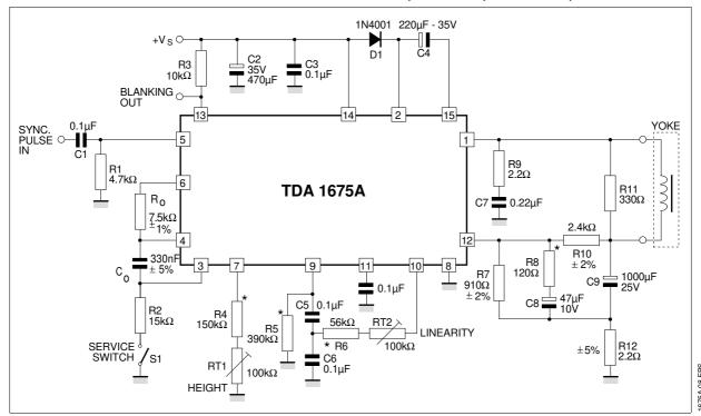
Figure 3 : Application Circuit for Small Scree  $90^{\circ}$  CTV Set (R<sub>y</sub> =  $15\Omega$  ; L<sub>y</sub> = 30 mH ; I<sub>y</sub> = 0.82 A<sub>PP</sub>)
