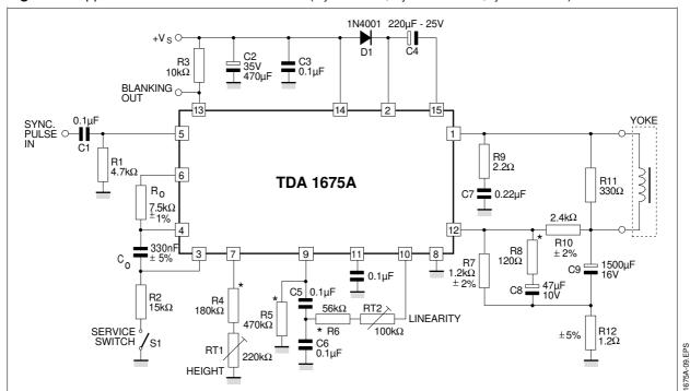
Figure 4 : Application Circuit for  $110^{\circ}$  CTV Set (R<sub>y</sub> =  $9.6\Omega$  ; L<sub>y</sub> = 24.6 mH ; I<sub>y</sub> = 1.2 A<sub>PP</sub>)
