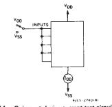
Fig. 14 - Quiescent-device current test circuit.
