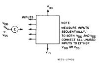
Fig. 16 - Input current test circuit.
