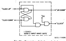
Fig. 11 – Conversion of clock up, clock down input signals to clock and up/down input signals.
