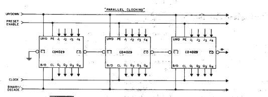
\* CARRY OUT lines at the 2nd, 3rd, etc., stages may have a negative-going glitch pulse resulting from differential delays of different CD4029B tC's. These negativegoing glitches do not affect proper CD4029B operation. However, if the CARRY OUT signals are used to trigger other edge-sensitive logic devices, such as FF's or counters, the CARRY OUT signals should be gated with the clock signal using a 2-input OR gate such as CD4071B.
