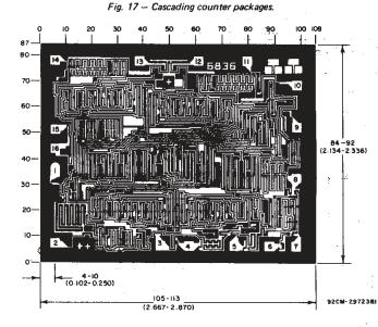
Chip dimensions and pad layout for CD4029B
