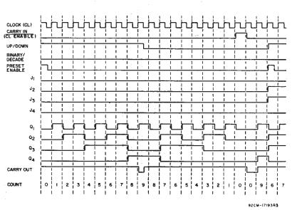
Fig. 12 - Timing diagram-decade mode.
