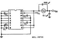
Fig. 13 - Power dissipation test circuit.
