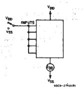
Fig. 29—Quiescent device current test circuit.
