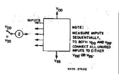
Fig. 31—Input-leakage-current test circuit.
