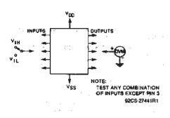
Fig. 30-input-voltage test circuit.
