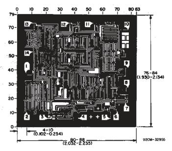
Chip dimensions and pad layout for CD4047B
