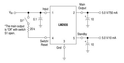
An input bypass capacitor is recommended if the regulator is located more than 4" from the supply input filter. The LM2935 is not internally compensated and thus requires an external output capacitor for stability. A minimum capacitance of 10  $\mu F$  is recommended. The actual capacitance value is dependent upon load current, temperature, and the capacitor's equivalent series resistance (ESR). The least stable condition is encountered at maximum load current and minimum ambient temperature.
