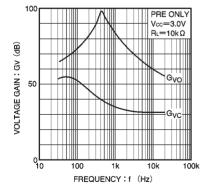
Fig. 24 Voltage gain vs. frequency
