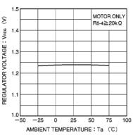
Fig. 28 Regulator voltage vs. ambient temperature
