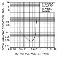
Fig. 23 Total harmonic distortion vs. output voltage
