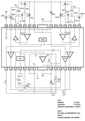
Fig. 8 Headphone stereo metal / normal switch
