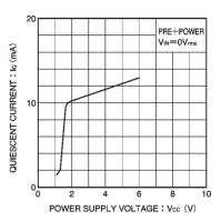
Fig. 20 Quiescent current vs. power supply voltage
