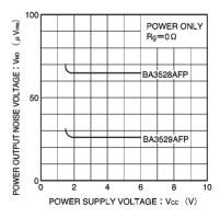
Fig. 26 Output noise voltage vs. power supply voltage
