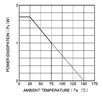
Fig. 18 Power dissipation vs. ambient temperature
