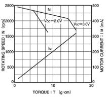
Fig. 29 Rotation speed and motor current vs. torque
