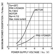
Fig. 19 Maximum power dissipation vs. power supply voltage
