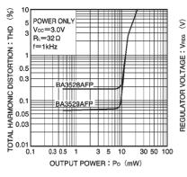
Fig. 27 Total harmonic distortion vs. output voltage
