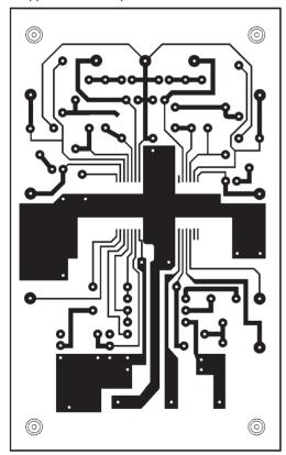
PCB thickness: 1.6mm Copper thickness: 35  $\mu$  m Copper side
