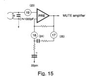
When countermeasures against strong electric fields for the power amplifiers are required, connect bypass capacitors between each input pin and pin 22, and connect choke coils in series with the output pins and the headphones. The component values should be about 330pF for the bypass capacitors, and the  $10\mu H$  for the choke coils so that they do not effect the audible frequency range.
