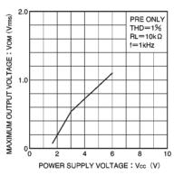
Fig. 22 Maximum output voltage vs. power supply voltage
