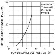
Fig. 25 Rated output power vs. power supply voltage
