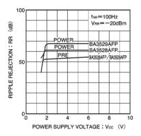
Fig. 21 Ripple rejection ratio vs. power supply voltage
