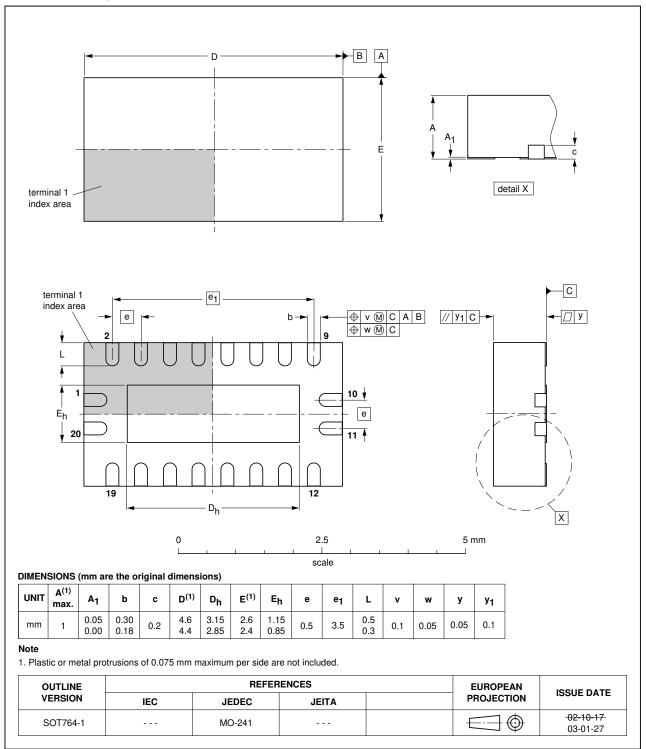
DHVQFN20: plastic dual in-line compatible thermal enhanced very thin quad flat package; no leads; 20 terminals; body 2.5 x 4.5 x 0.85 mm SOT764-1
