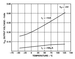
Figure 14. Output Voltage Swing vs. Temperature
