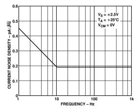
Figure 28. Input Bias Current Noise Density vs. Frequency
