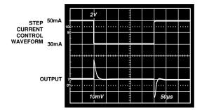
Figure 45. Output Step Load Current Recovery
