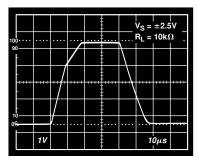
Figure 33. Large Signal Transient Response
