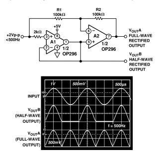
Figure 42. Single-Supply Half-Wave and Full-Wave Rectifiers Using an OP296
