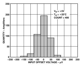
Figure 2. Input Offset Voltage Distribution
