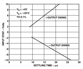
Figure 29. Settling Time to 0.1% vs. Step Size
