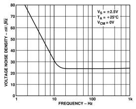
Figure 27. Voltage Noise Density vs. Frequency
