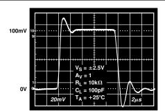
Figure 31. Small Signal Transient Response
