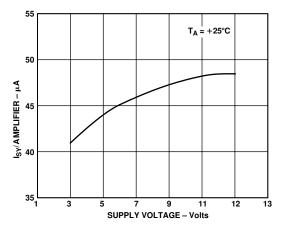
Figure 26. Supply Current/Amplifier vs. Supply Voltage
