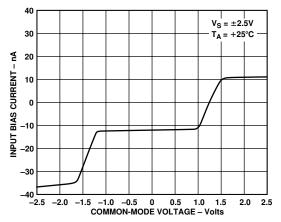
Figure 9. Input Bias Current vs. Common-Mode Voltage
