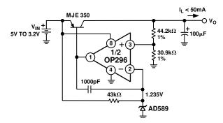
Figure 44. 3 V Low Dropout Voltage Regulator
