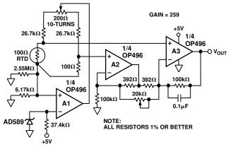
Figure 48. A Single Supply RTD Amplifier
