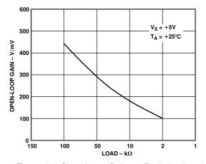
Figure 19. Open Loop Gain vs. Resistive Load
