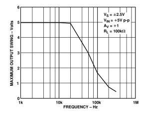
Figure 24. Maximum Output Swing vs. Frequency
