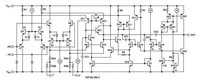
Figure 36. Simplified Schematic
