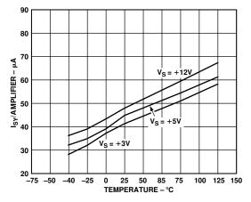
Figure 25. Supply Current/Amplifier vs. Temperature
