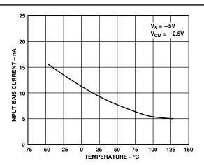
Figure 7. Input Bias Current vs. Temperature
