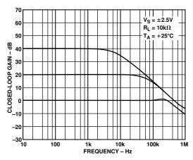
Figure 20. Closed-Loop Gain vs. Frequency
