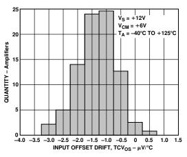
Figure 5. Input Offset Voltage Distribution (TCV<sub>OS</sub>)
