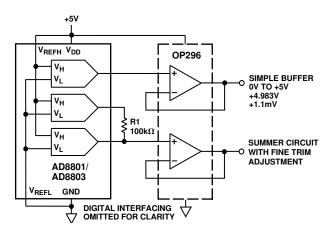
Figure 46. Buffering a TrimDAC Output
