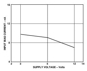
Figure 8. Input Bias Current vs. Supply Voltage
