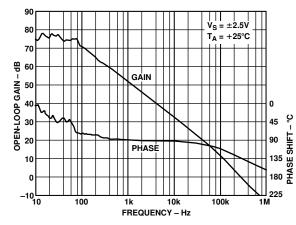
Figure 15. Open-Loop Gain and Phase vs. Frequency (No Load)
