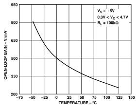
Figure 18. Open-Loop Gain vs. Temperature
