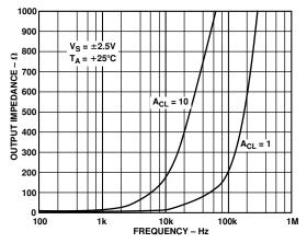
Figure 21. Output Impedance vs. Frequency
