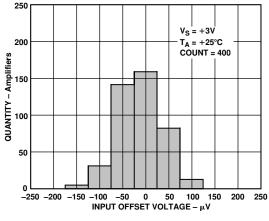
Figure 1. Input Offset Voltage Distribution
