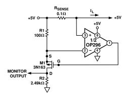
Figure 47. A High-Side Load Current Monitor
