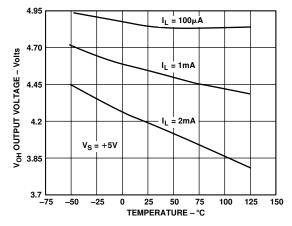
Figure 13. Output Voltage Swing vs. Temperature
