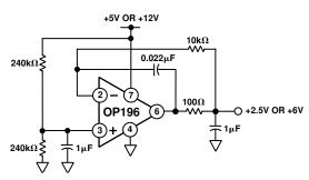
Figure 41. A Micropower False-Ground Generator
