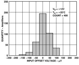
Figure 3. Input Offset Voltage Distribution
