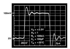
Figure 32. Small Signal Transient Response
