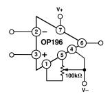
Figure 39. Offset Nulling Circuit
