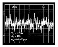
Figure 30. 0.1 Hz to 10 Hz Noise
