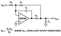
$C_{F} = \left[ I + \left( \frac{I}{|A_{CL}|} \right) \right] \left( \frac{R_{F} + R_{G}}{R_{F}} \right) C_{L} R_{O}$
