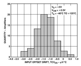
Figure 4. Input Offset Voltage Distribution (TCV<sub>OS</sub>)
