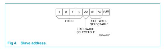
The last bit of the slave address defines the operation to be performed. When set to logic 1, a read operation is selected, while a logic 0 selects a write operation.
