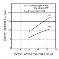
Fig.2 Current dissipation 2,3 vs. power supply voltage
