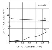
Fig.3 Output voltage vs. output current
