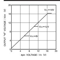
Fig.4 Output voltage vs. 4 pin voltage
