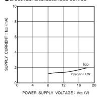
Fig.1 Current dissipation 1 vs. power supply voltage
