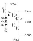
1) When the output voltage control pin (pin 4) is used  $V_R < V_{CC1} - (V_{SAT (Q1)} + V_{BE (Q5)} + V_{BE (Q6)} + V_{BE (Q7)}) = V_{CC1} - 2.5V$
