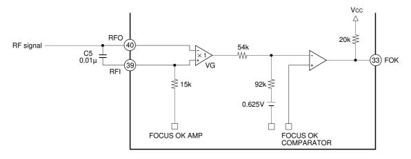
The focus OK circuit creates the timing window okaying the focus servo from the focus search state.
