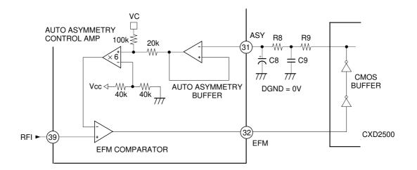
As this comparator is a current SW type, each of the High and Low levels is not equal to the power supply voltage. A feedback has to be applied through the CMOS buffer.
