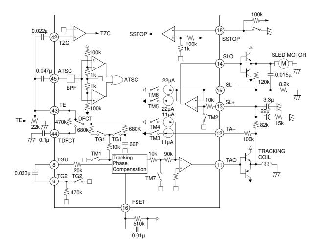
The above figure shows a block diagram of the tracking and sled servo.
