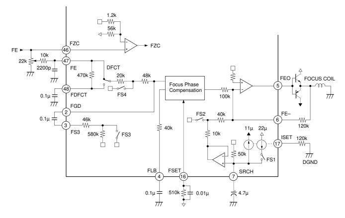
The above figure shows a block diagram of the focus servo.
