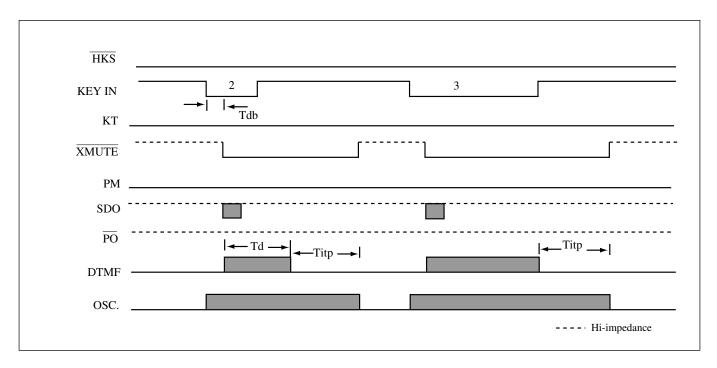
Figure 2. DTMF mode operating timing
