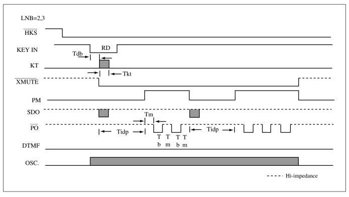
Figure 3. Pulse mode LNB redial timing
