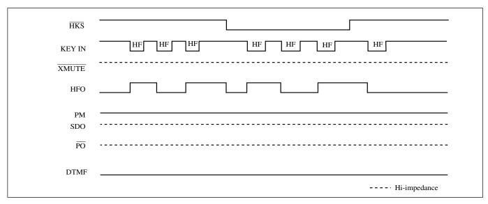
Figure 9. HF operating timing
