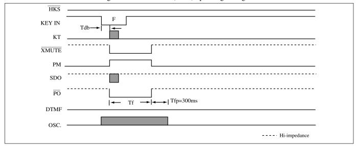
Figure 7. Flash key operating timing
