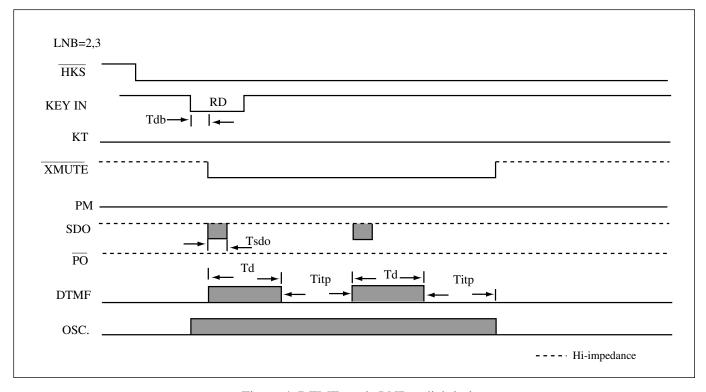
Figure 4. DTMF mode LNB redial timing
