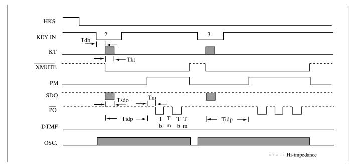
Figure 1. Pulse mode operating timing
