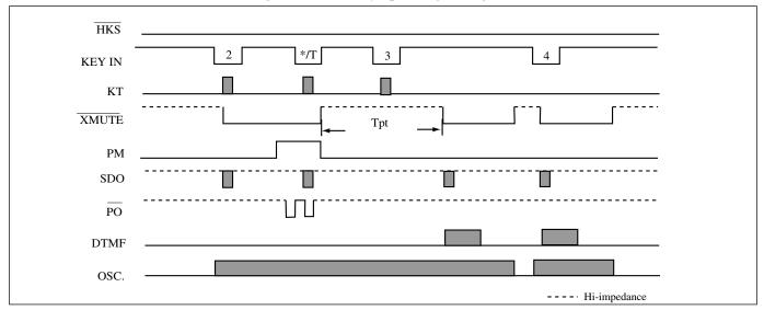
Figure 6. Pulse to Tone  $(P \rightarrow T)$  operating timing
