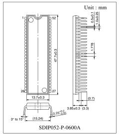
Note) The package of this product will be changed to lead-free type (SDIP052-P-0600F). See the new package dimensions section later of this datasheet.
