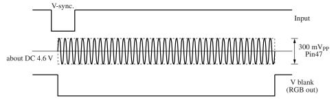
Note) \*2: Eventhough the MICOM switches the VCO between 4.43MHz and 3.58MHz, only the 4.43 MHz CW will be outputed at periodic intervals as shown below.
