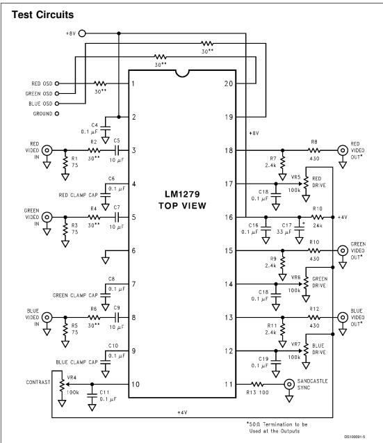
\*\*Note: All video inputs must have a series  $30\Omega$  resistor for protection against EOS (Electrical Over Stress). If the OSD signals are external to the monitor, or these signals are present any time when +8V is not fully powered up, then the OSD inputs also require a series  $30\Omega$  resistor.
