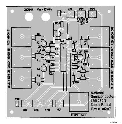
FIGURE 7. LM1279 OSD Video Pre-Åmp Demontration Board Layout
