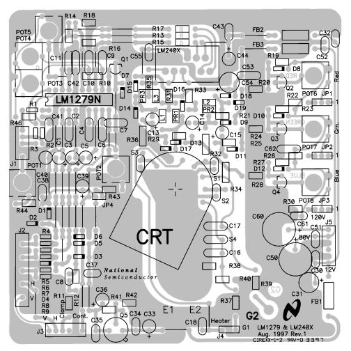
FIGURE 11. LM1279/LM2407 Demonstration Neck Board Layout
