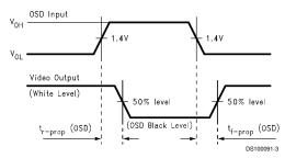
FIGURE 3. OSD Propagation Delays
