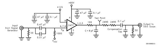
Note: 8 pF load includes parasitic capacitance.
