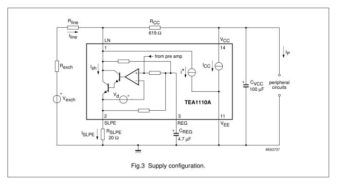
The internal circuitry of the TEA1110A is supplied from pin  $V_{CC}$ . This voltage supply is derived from the line voltage by means of a resistor ( $R_{CC}$ ) and must be decoupled by a capacitor  $C_{VCC}$ . It may also be used to supply peripheral circuits such as dialling or control circuits. The  $V_{CC}$  voltage depends on the current consumed by the IC and the peripheral circuits as shown by the formula:
