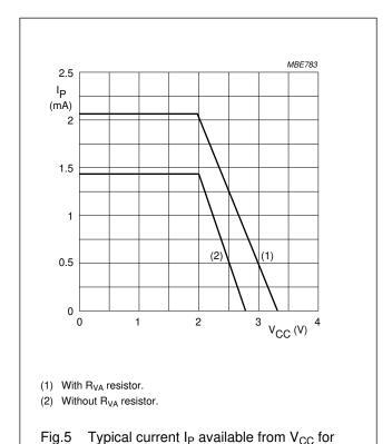
peripheral circuits at I<sub>line</sub> = 15 mA.
