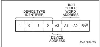
The next bit addresses a particular device. A system could have up to two X24C08 devices on the bus (see Figure 10). The two addresses are defined by the state of the A2 input.
