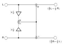
The structure of the matrix surround is as shown in the figure above. Use the equations shown in the figure to calculate gain.
