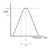
1) The BPF is composed of a multifeedback active filter.  $f_{\circ}$  can be varied according to the value of C. (theoretical equation)
