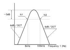
Cutoff frequency (fc1) for the bypass filter can be changed using the attached C1.
