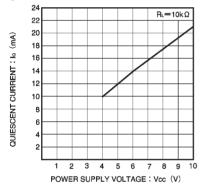
Fig. 3 Quiescent curve vs.power supply voltage
