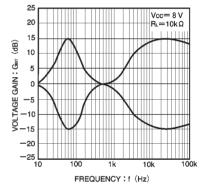
Fig. 5 Output gain vs.frequency
