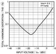
Fig. 4 Harmonic distortion vs.input voltage
