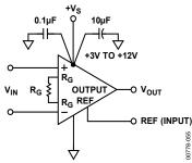
Figure 43. Single-Supply Basic Connection
