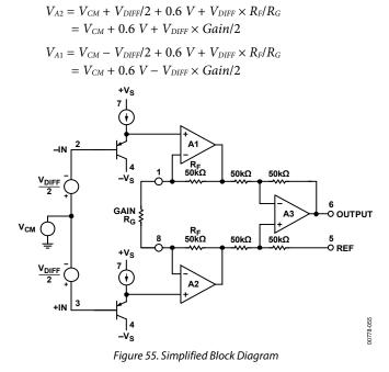
The voltages on these internal nodes are critical in determining whether the output voltage is clipped. The  $V_{A1}$  and  $V_{A2}$  voltages can swing from approximately 10 mV above the negative supply (V– or ground) to within approximately 100 mV of the positive rail before clipping occurs. Based on this and from the previous
