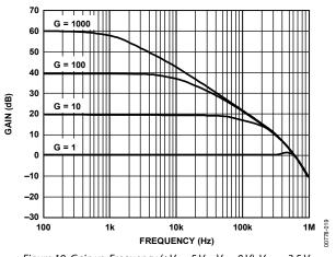
Figure 19. Gain vs. Frequency  $(+V_s = 5 V, -V_s = 0 V)$ ,  $V_{REF} = 2.5 V$ , for Various Gain Settings (G)
