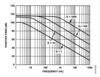
Figure 25. Positive PSRR vs. Frequency,  $+V_5 = 5V$ ,  $-V_5 = 0V$ , for Various Gain Settings (G)
