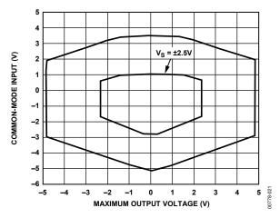
Figure 21. Maximum Output Voltage vs. Common-Mode Input,  $G \ge 10$ ,  $R_L = 100 \Omega$ , for Two Supply Voltages
