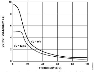
Figure 27. Large Signal Response,  $G \le 10$  for Two Supply Voltages
