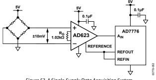
Figure 53. A Single-Supply Data Acquisition System
