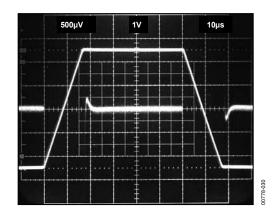
Figure 30. Large Signal Pulse Response and Settling Time, G = -10 (0.250 mV = 0.01%),  $C_L = 100 \text{ pF}$
