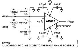
Figure 45. Circuit to Attenuate RF Interference
