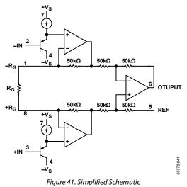
Because of the voltage feedback topology of the internal op amps, the bandwidth of the in-amp decreases with increasing gain. At unity gain, the output amplifier limits the bandwidth.
