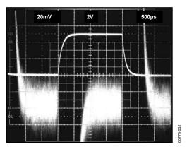
Figure 32. Large Signal Pulse Response and Settling Time, G = -1000 (5 mV = 0.01%),  $C_L = 100 \, pF$
