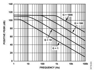
Figure 24. Positive PSRR vs. Frequency
