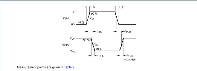
$\ensuremath{V_{\text{OL}}}$  and  $\ensuremath{V_{\text{OH}}}$  are typical output voltage levels that occur with the output load.
