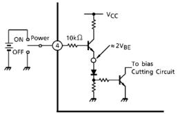
Fig.3 With pin(4) set to high, power is turened on.
