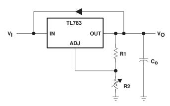
Figure 15. Regulator With Protective Diode
