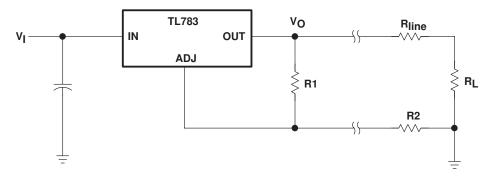
Figure 16. Regulator With Current-Set Resistor
