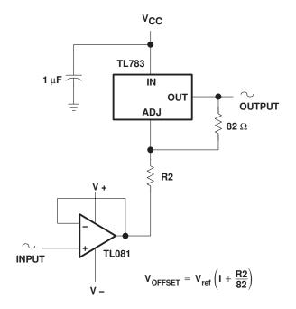
Figure 23. High-Voltage Unity-Gain Offset Amplifier
