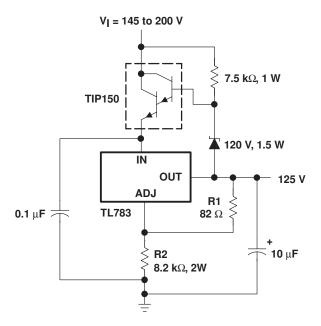
Figure 18. 125-V Short-Circuit-Protected Off-Line Regulator
