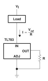
Figure 21. Current-Sinking Regulator
