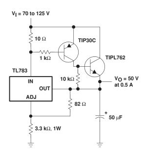
Figure 19. 50-V Regulator With Current Boost
