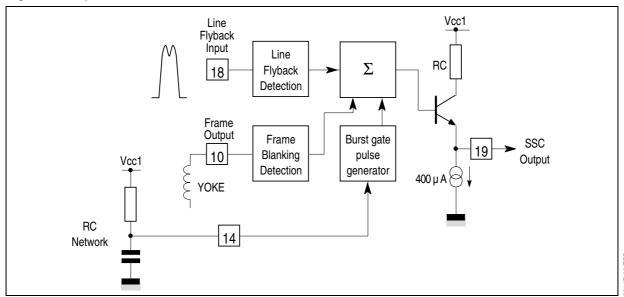
Figure 8: Video Identification Circuit (Pin 8)
