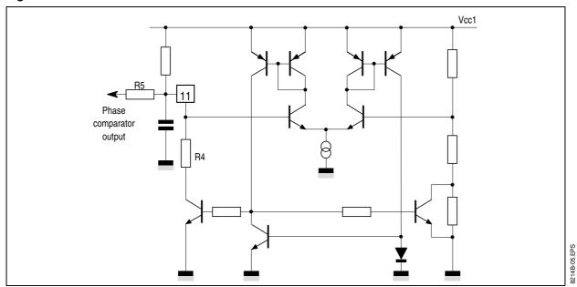
The oscillator thresholds are internally fixed by resistors. The discharge of the capacitor depends on the internal resistor R4. The control voltage is applied on resistor R5.
