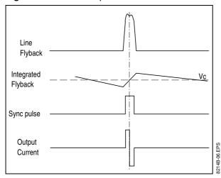
The sync-pulse drives the current in the comparator. The line flyback integrated by the external net work gives on pin 13 a saw tooth, the DC offset of this saw tooth is fixed by VC. The comparator output provides a positive current for the part of the signal on pin 13 greater than to VC and a negative current for the other part. When the line flyback and the video signal are synchronized, the output of the
