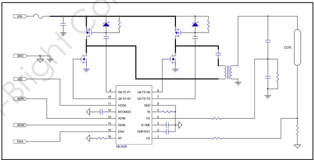
Figure 1: OB3328 Typical Application Schematic
