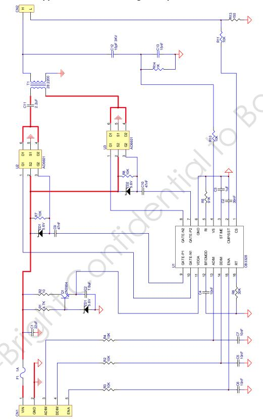
VIN: 8~22V ADIM: 3V, Max. Brightness; 0V, Min. Brightness (for analog mode dimming) DDIM: 3V, Max. Brightness; 0V, Min. Brightness (for burst mode dimming) ENA: Disable, 0-0.8V; Enable, 2-5V LOAD: 82.5Kohm Dummy Load
