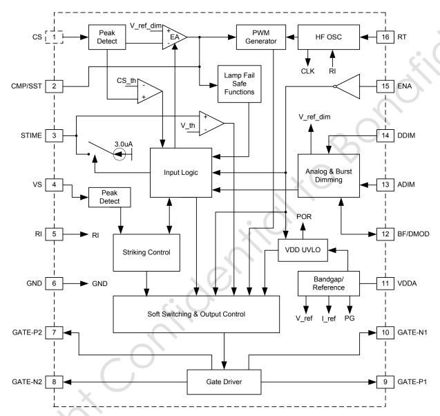
Figure 2: OB3328 Functional Block Diagram
